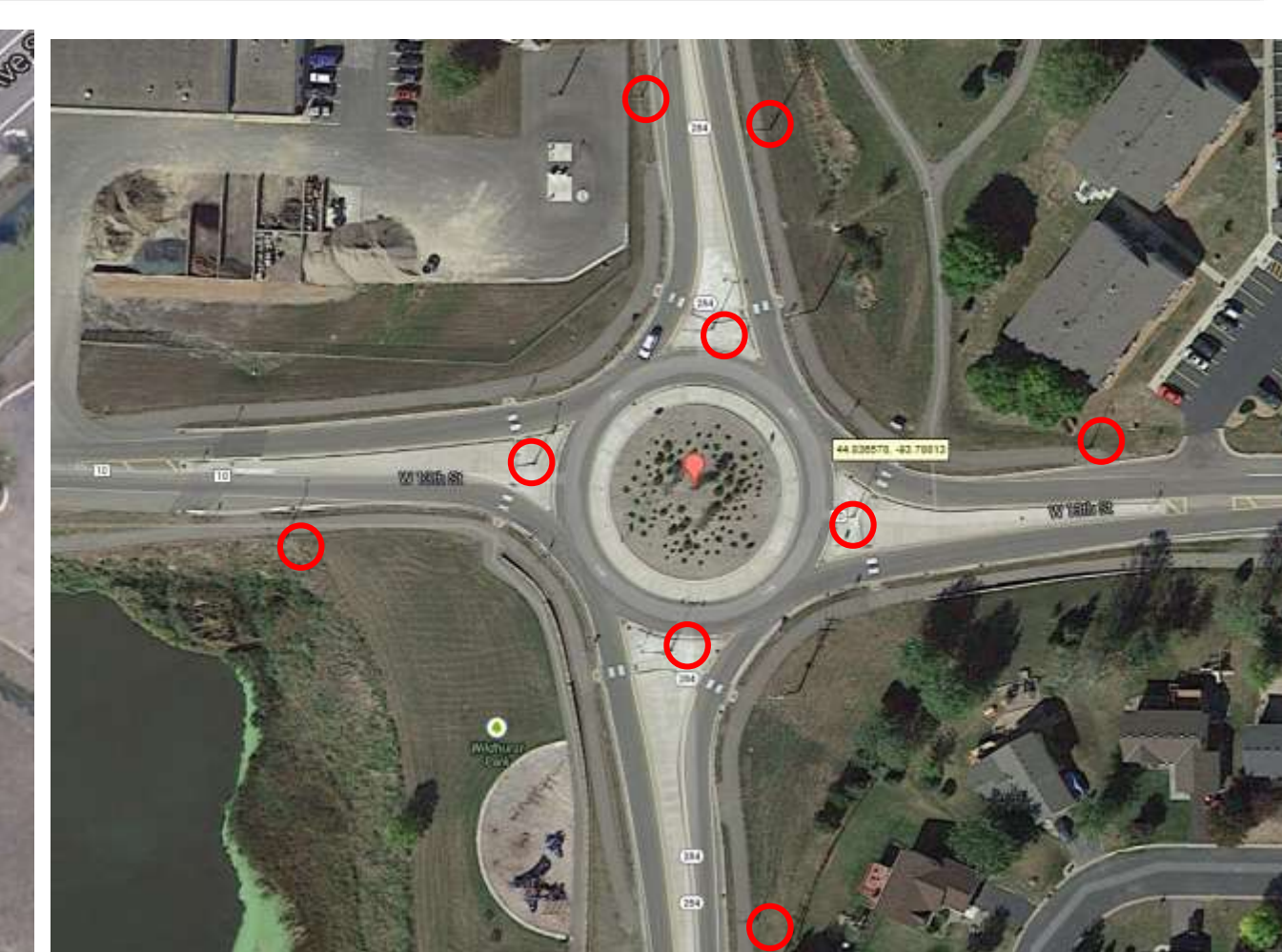
Typical Roundabout "Full" Illumination Layout in MN
